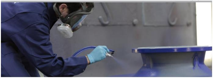
We now offer efficient cartridge application for some selected products. We decided to implement the advanced Mixpac technology from the company Sulzer to simplify the complex coating application procedure significantly. An optimum solution for repairs, small projects or areas which are difficult to access!
