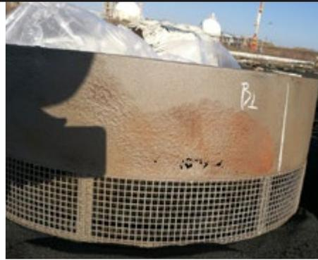
Previous condition: The whole motor showed corrosion damages. On connection box and impeller housing severe pitting corrosion occurred. 4 motors in total are installed in this plant, the first has now been renovated with our systems.
