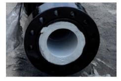
After full curing, the surface was inspected with an electronic spark detector (Holiday tester, high voltage 3 kV – according to NACE guidelines). No pinholes, blistering ore cracks were detected, the coating material showed a smooth surface. The specification required a total layer thickness of  $1000\mu m$ , which was also tested thoroughly.
