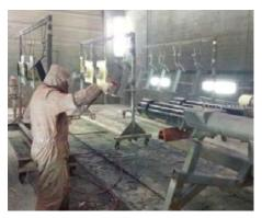
The shaft and the paddle construction are placed in the variable range of biogas and biomass. The steel components are steadily exposed to the influences of the biogas, which provoke the highly corrosive effect. A coating system with excellent physical properties and resistances is essential for this kind of application.
