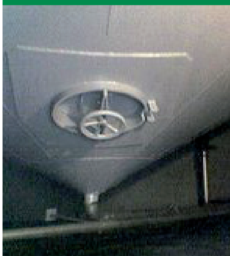
Fermentation tank after renewal with Proguard CN 200
