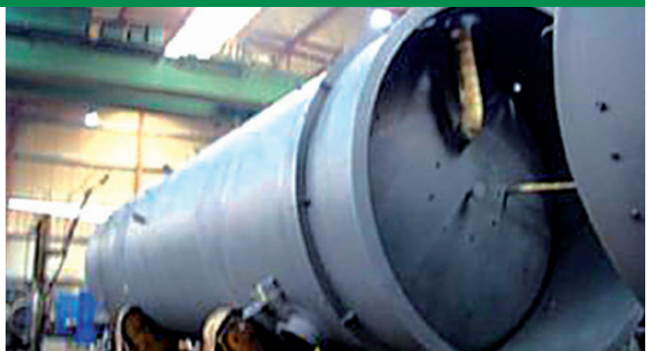
Internal coating of huge hot-water tanks
