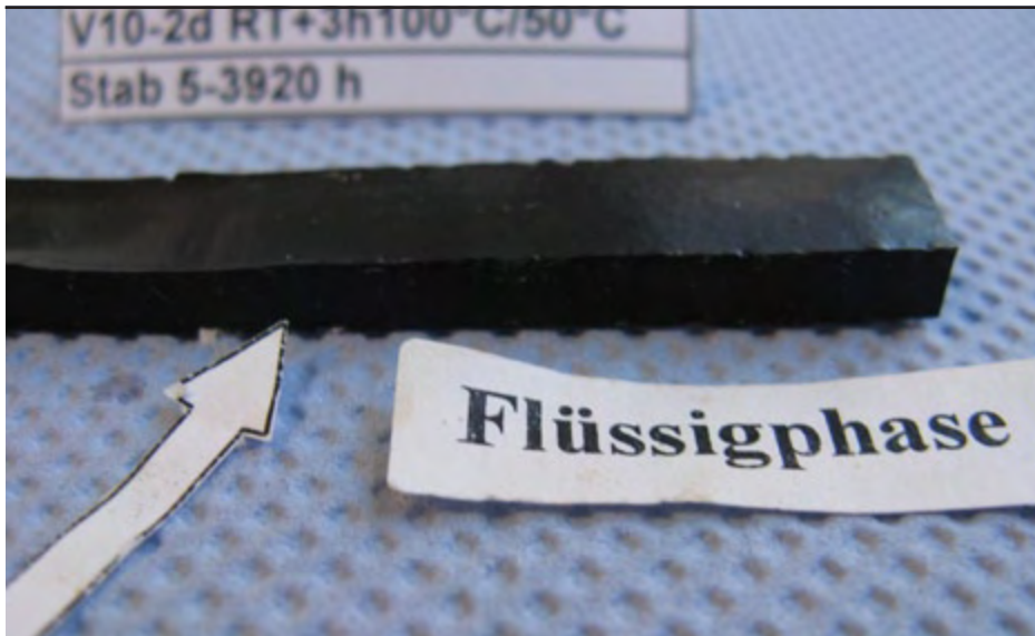
Proguard CN-1M test rod after 3.920 hours of storage in the highly aggressive test-liquid
