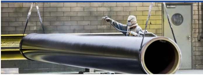
"Wintershall" is the biggest international operating German company for the oil and gas production. For an oil platform in the North Sea, 16 huge casing pipes for the demanding area of splash zone and fluctuating water level were coated with our product CERAMIC-POLYMER SF/LF-3. The application of the coating was professionally conducted by "De Back Metaalconservering Groep", our partner for the Netherlands.
