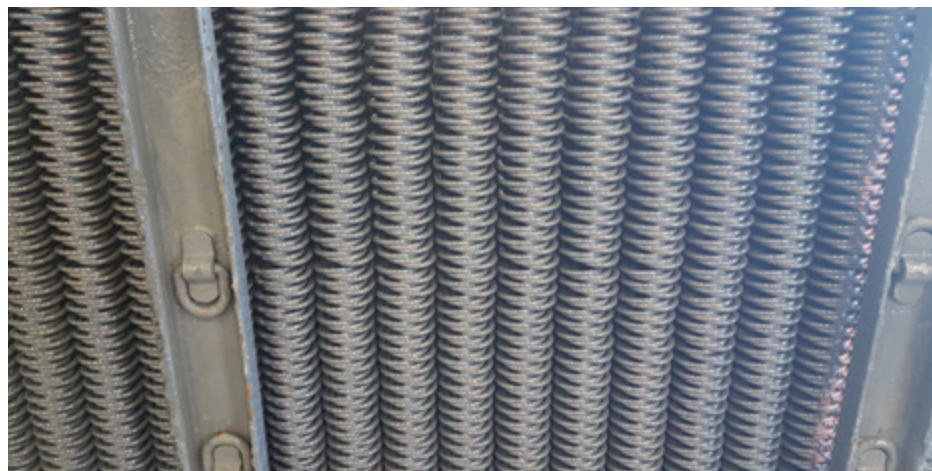
After flooding all loops of the cooler are durably protected against corrosion and dirt deposits.
