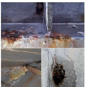
After 2 years of service severe pitting corrosion was detected especially at corners and edges of the stainless steel tanks. The 33 % solution of sodium chloride and water in combination with the elevated operation temperature of 45 °C is an excessively high chemical load for long-term use – even for stainless steel substrates.
